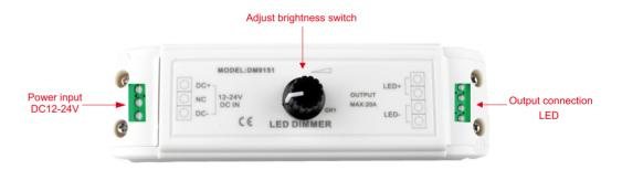
As Shown, the LED load and power's negative and positive with the right interface, open the power supply, regulator potentiometer, so as to change the output of the controller, until getting the satisfactory of LED output. Potentiometer with switch function, when shutdown controller will cut off power supply.
