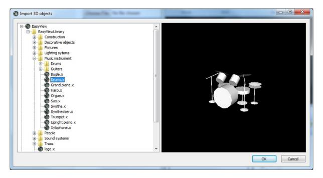
The library on the left side displays the available objects to be inserted. Once selected, the object automatically appears in the visualization window. The object selected may be previewed before it is inserted. Click on "Select" to insert the object in your stage.
